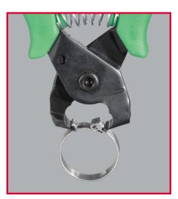
Nose of the pliers should be firmly seated under the assembly bump and lock latch.
