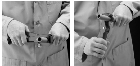
The rotating/rocking technique produces fast easy cuts.
