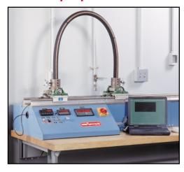
With standard SAE impulse performance of 500,000 cycles at one-half bend to one million cycles at full SAE bend radii, Aeroquip's new FC659 is the future of high pressure hose.
