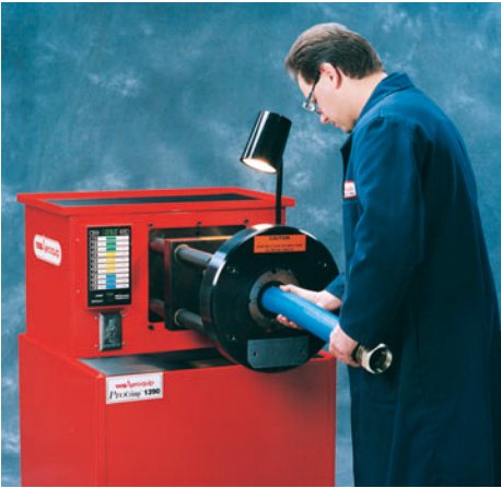
ProCrimp 1390 can be activated by foot pedal or hand operated switch.
