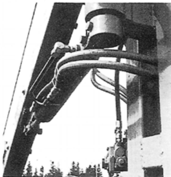
Fig. 1. In flexing applications, the hose assembly should be routed through the pivot point around which the component is moving.
