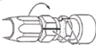
Misalignment of the mark shows the amount which the nut was tightened.
