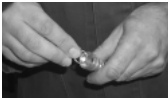
Figure 5 - Braze ring installation
