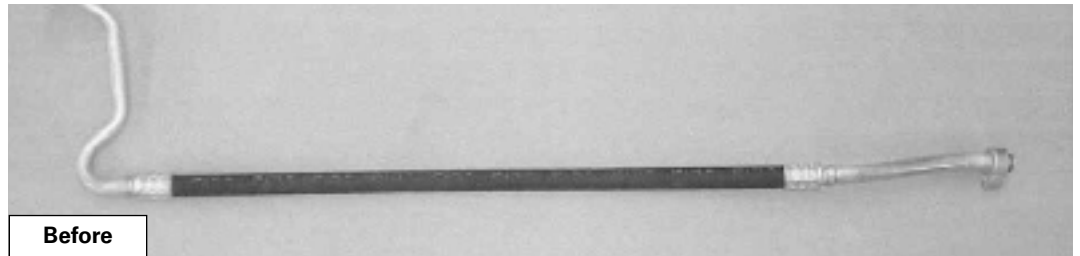
Figure 1. Failed Hose Assembly. Note crimp fittings.
