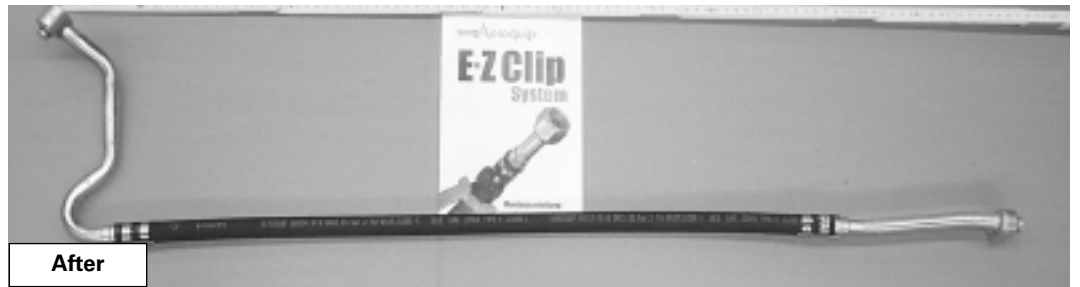
Figure 2. Completed hose assembly. Note E-Z Clip Fittings.
