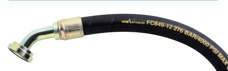
Eaton's new FC849 family of hose offers 4,000 psi operating pressure in every size. Featuring a compact design plus superior flexibility, it's available in sizes -4 through -12. This new easy-to-route product is qualified for use with Aeroquip's global skive and global Through-The-Cover crimp fittings. FC849 hose routes easily, reducing hose length requirements. By having only one part number in inventory, selection is greatly simplified.
