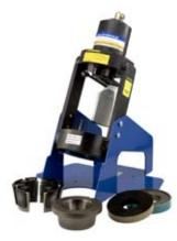
The completely PORTABLE ET1000 crimp machine boasts a broad crimp capability with an ease-of-use that is sure to please hose assemblers. With 3 power source options - air/hydraulic, hand and electric - this portable machine can travel to the work-site. The machine comes equipped with a stand pre-drilled for mounting to a work-bench or table-top.
