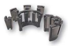
The two-piece caged style fits easily into the palm of the hand for quick and easy transfer of collets. The eightsegment design creates a full 360° crimp and features a replaceable cage. The larger 1-1/2" and 2" size collets are vulcanized (no cage) for easier handling.
