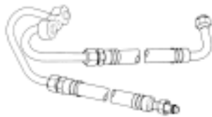
Typical assembly of a flareless hose end used with an old original equipment end configuration.
