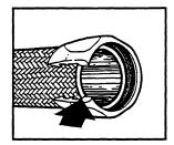
Step 2. Insert hose in socket with twisting, pushing motion until hose is in line with back of the socket threads.
