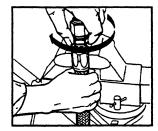
Step 4. Carefully insert nipple and engage nipple and socket threads while holding hose in position with other hand. Make sure hose does not push out of socket.
