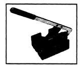
Step 1. Cut hose square to length with Aeroquip cut off tool (FT1258) or similar cutting device.
