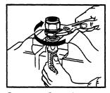
Step 5. Complete assembly using wrench while continuing to hold hose in position.
