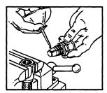
Step 3. Lubricate inside of hose and nipple threads liberally using S.A.E. 30 lubricating oil or Aeroquip FBM3553 hose assembly lube.
