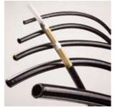
At its core, Synflex® High Pressure Hose is a smooth, seamless, continuous extrusion of Nylon 11 Besno P40TLO. The hose is reinforced with aramid (Kevlar®) fiber and jacketed with highly UV resistant thermoplastic for long term
