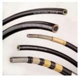
Synflex<sup>®</sup> Subsea HCR Collapse Proof Hoses are reinforced with aramid (Kevlar<sup>®</sup>) fiber bonded to the core tube and cover. The tube is a smooth, seamless, continuous extrusion of Besno Nylon 11 P40TLO, and the flexible 316 stainless
