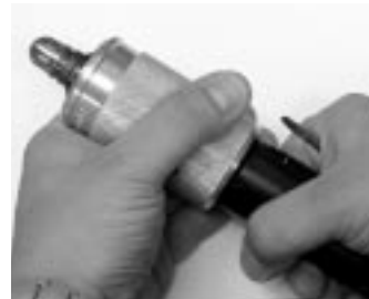
Figure 3 – Twisting Tool To Release
